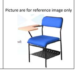
provided under the seat. The frame structure shall be supported by four legs made up of MS/CRCA powder coated round pipe of 1.5mm thick. There shall be PPCP shoe provided at the base to avoid scratches on the floor. The seat size shall be 410±10 mm(D) X 415±10 mm(W) and back size shall be 460±10 mm(W) X 300±10 mm(H) from seat. Overall height shall be = 770±10 mm.
